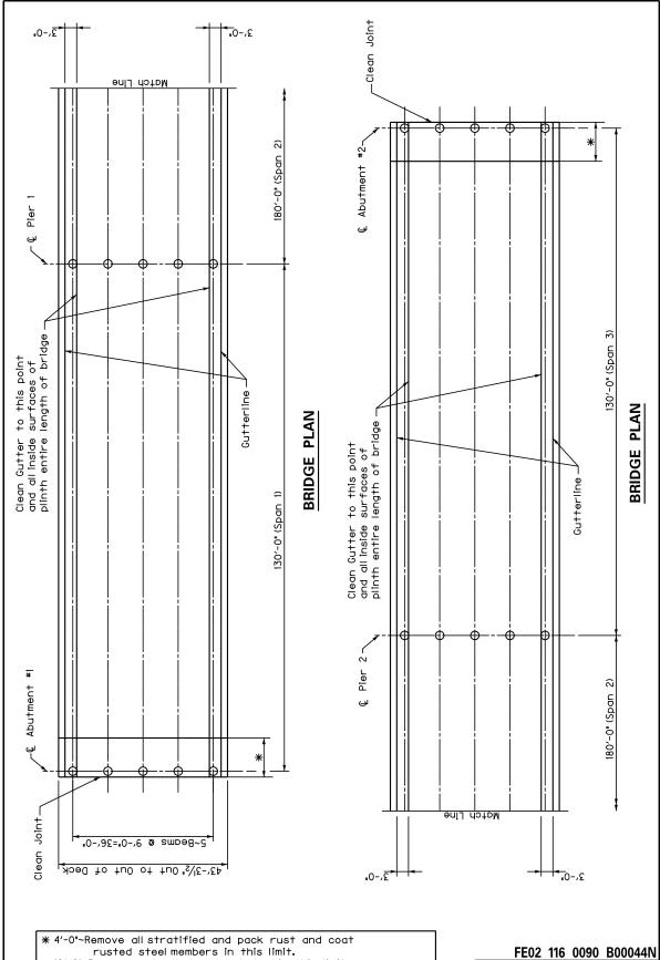
rusted steel members in this limit. 10'-0"~Presserwash all structural steel in this limit. O Indicates bearings to be greased, 20 total. Remove Debris, Pressure Wash and apply concrete sealant at all substructrue units. See Secial Note for Bridge Cleaning and Preventive Maintenance.
