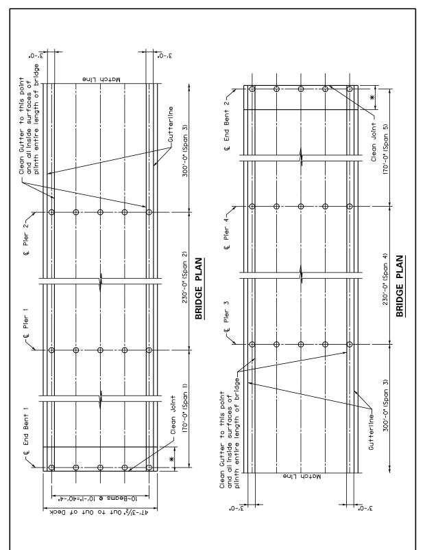
\* 4'-0'~Remove all stratified and pack rust and coat rusted steel members in this limit.
