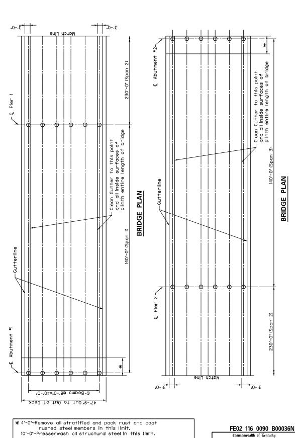
O Indicates bearings to be greased, 24 total. Remove Debris, Pressure Wash and apply concrete sealant at all substructrue units. See Secial Note for Bridge Cleaning and Preventive Maintenance.
